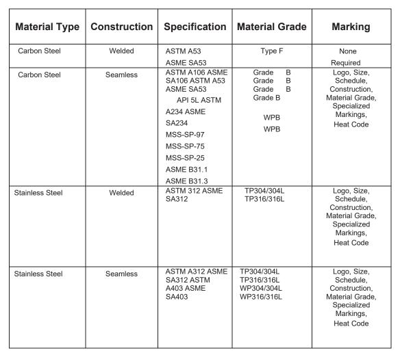
Close and short nipples, along with some of the small diameter nipples, bull plugs and swages are packed in labeled boxes and may not carry the marking shown above due to space limitations. Additionally, some information may be abbreviated or omitted by the guidelines shown in MSS SP-25. All marking is performed with low-stress stamps for both carbon and stainless grades.
